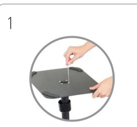
Position base plate over aluminium collar of bottom post, ensuring the two rivets (marked X) point towards the 7mm security cord slot. Insert and tighten 4 base plate screws to secure.
