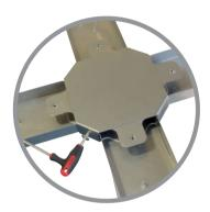
Carefully position and lower octagonal centre cover onto bottom support plate. Align two side holes of cover to any thread fixings of bottom support plate. Insert and tighten two hex socket screws to secure octagonal centre cover.
