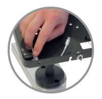
Lift fascia out of enclosures. Insert cables (supplied with Apple iPad) into all holders, allowing 10cm to remain "free" at charge/sync connector end by gently pressing into retaining moulding.
