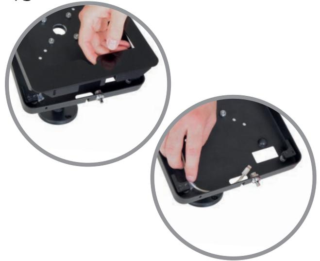
Lift fascia out of enclosure. Insert cable (supplied with Apple iPad) allowing 10cm to remain "free" at charge/sync connector end by gently pressing into retaining moulding.
