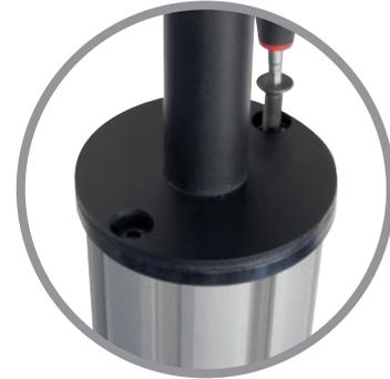
Align first 2 holes of the iPad holder to the threads of the post. Insert and tighten screws to secure. Rotate iPad holder through 90°, aligning remaining 2 holes to threads of post. Insert and tighten screws to secure.
