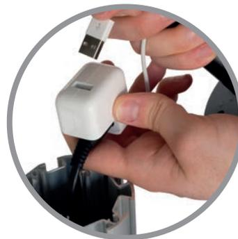
Plug cable into USB Power Adapter.
