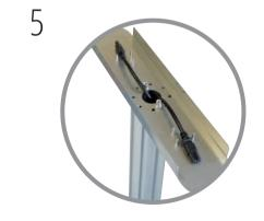
Feed figure 8 heads of power lead through central hole of bottom support plate and carefully place plate onto post. Align 4 holes to threads inside post at desired display angle.
