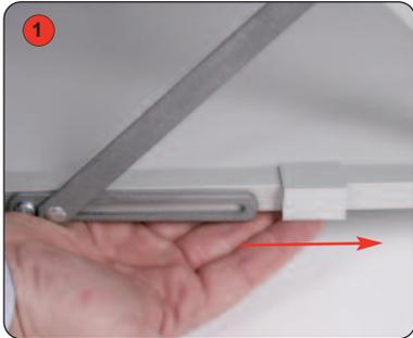
Slide locking tab away from pivot arm at base of unit. Repeat for 2nd locking tab.
